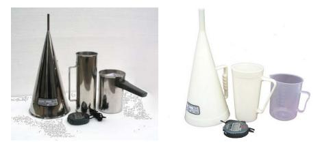
The MKW-MFV Marsh Funnel Viscometer is an easy to use apparatus used to measure the viscosity of drilling fluids. The relative viscosity of the drilling fluid can be measured by this sturdy and heat resistant march funnel. Simply record the number of seconds required for a given volume of drilling fluid to pass through the marsh funnel.
